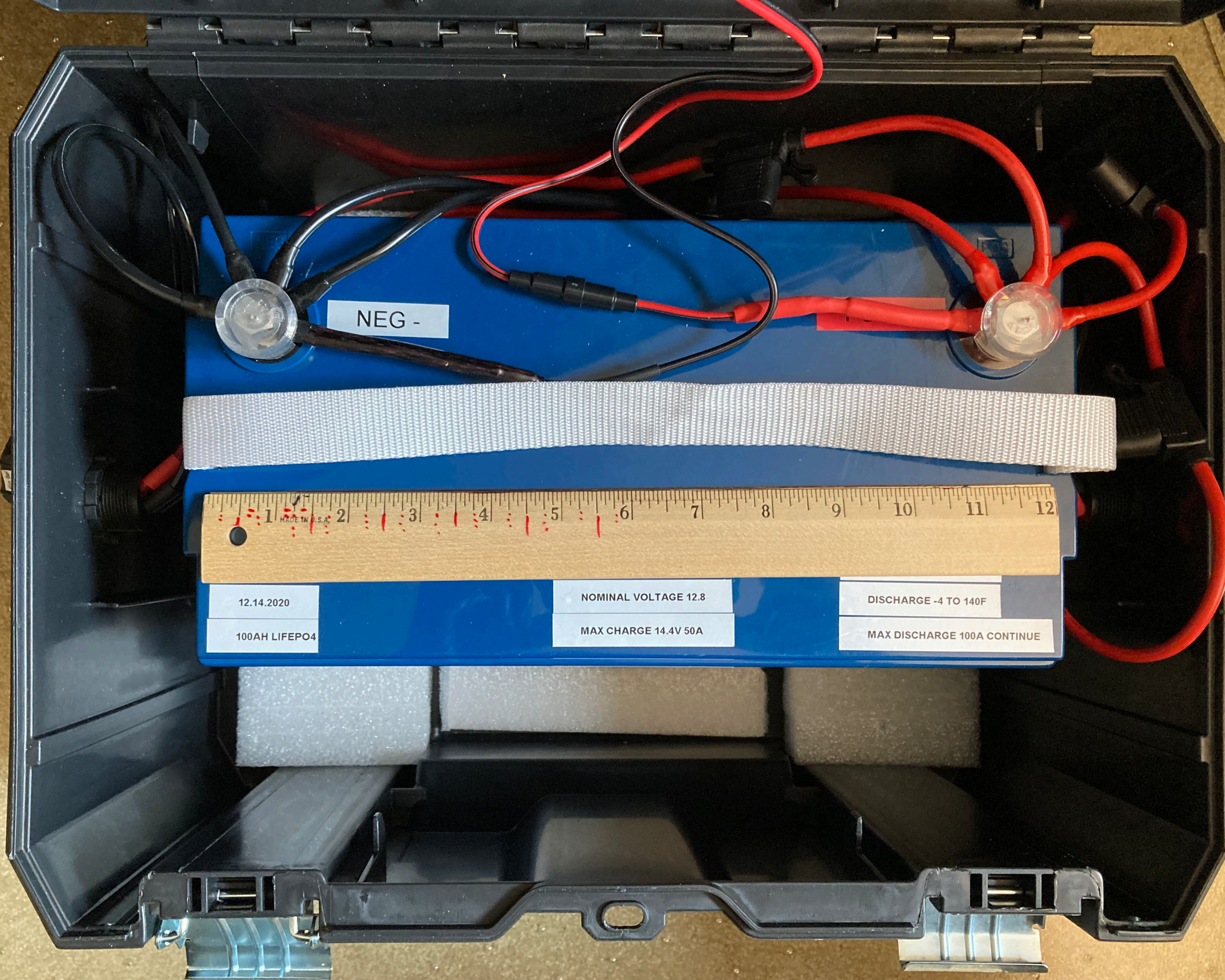
100AH LFP BATTERY IN LARGE, DEWALT TOOL BOX. BATTERY REQUIRES TALL BOX TO FIT.
