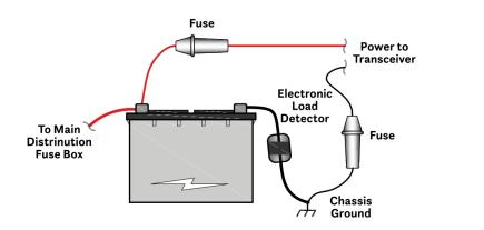
When powering your mobile radio by connecting it directly to the vehicle's battery, place the fuses as close to the battery as possible. In the event that the current draw is higher than the value of the fuse, the fuse will do its job and break the circuit.
