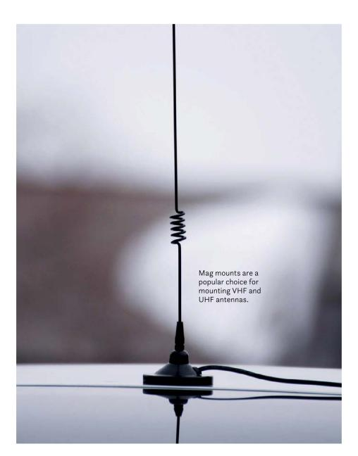
HF antennas are generally large and heavy, with a lot of wind resistance, so you should avoid using a mag mount in these types of installations. As a rule, for best performance and safety, HF antennas should use a solid physical mount with a good ground connection.
