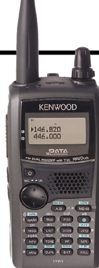
The Kenwood TH-D72 is an example of a feature-rich analog-only transceiver.
