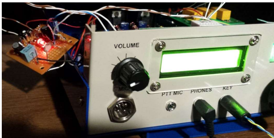
Figure 3. The AGC circuit is assembled on a small board and wired directly to the volume control.
