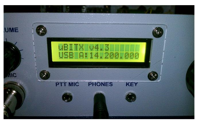
In order to calibrate your Micro-BITX, you need to be able to connect your radio to an antenna, and tune in a signal with a known frequency. Time and frequency standards stations such as WWV (5.0, 10.0, 15.0, and 20.0 MHz) or CHU (3.33, 7.85, and 14.67 MHz) are good choices. You can also use a shortwave broadcast station, but you may find them more difficult to tune in when they're broadcasting music. I like using WWV.
