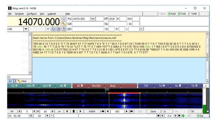
My radio display read a bit high – 15.000.050. Pretty close. The 600 Hz tone I should have been receiving was also at actually 592 Hz. Let's see if we can get the calibration closer. I turned the VFO to read 15.000.000 MHz, then entered the calibration menu to make an adjustment.
