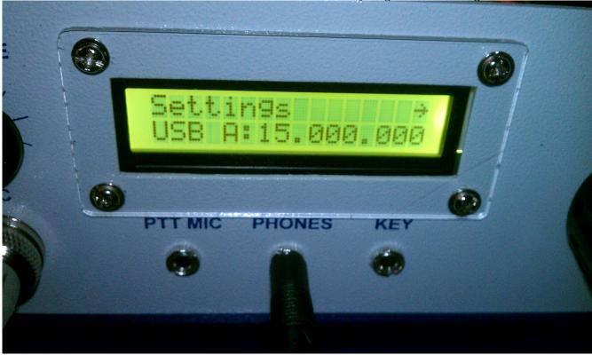
Press the VFO knob. The top line of the LCD will briefly display a "Settings On" message, then show the calibrate menu below. Note: you will be able to enter the settings menu again and make changes until you either turn the settings menu back off again, or you remove power from the radio.
