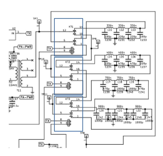
The stock low Pass Filter inputs and outputs for each frequency range are routed through the same, small relay. Capacitive coupling between the relay structures is limiting the effectiveness of the filters.
