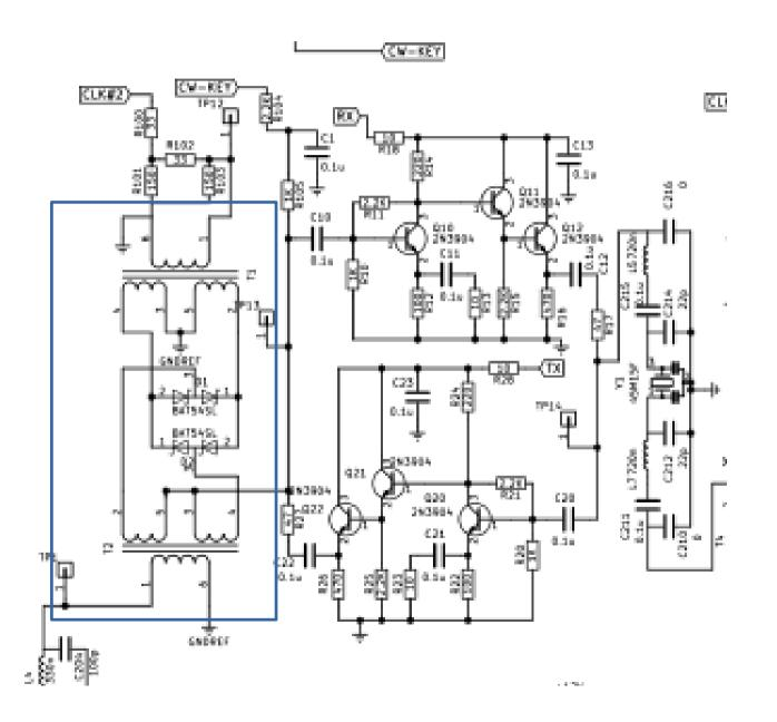
The stock 45 MHz Transmit Mixer is picking up RF energy from the transmitter final amplifier, and is being overloaded, resulting in spurs.
