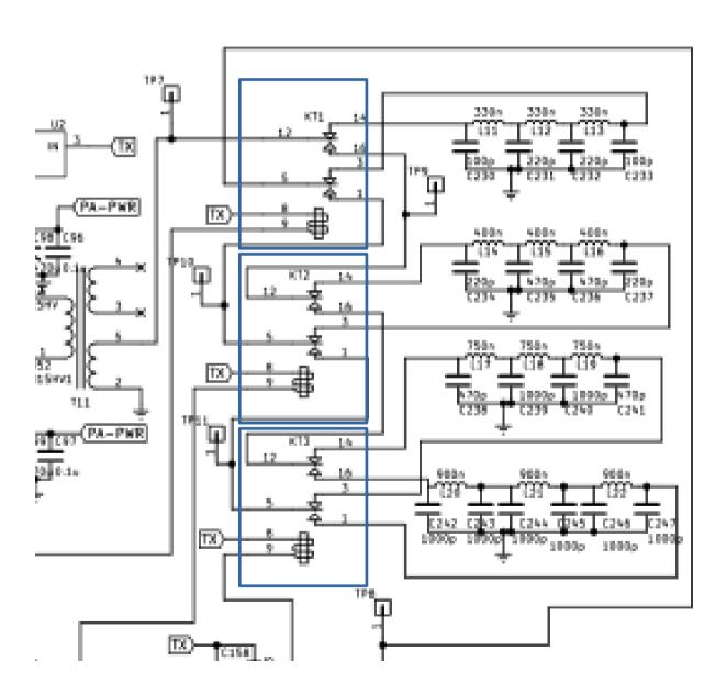
Currently, the low Pass Filter inputs and outputs for each frequency range are routed through the same, small relay. Capacitive coupling between the relay structures is limiting the effectiveness of the filters.
