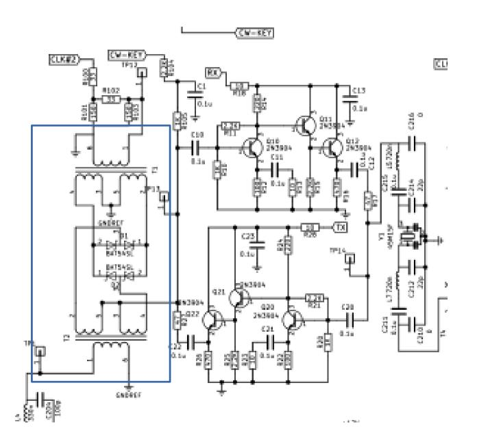
45 MHz Transmit Mixer is picking up RF energy from the transmitter final amplifier, and is being overloaded, resulting in spurs.
